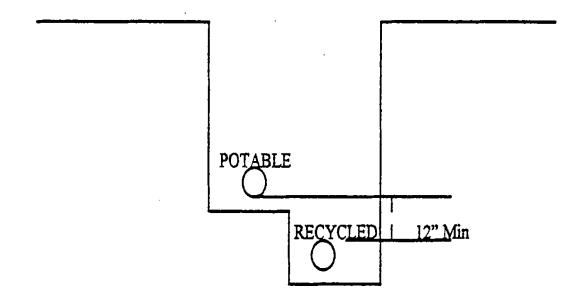
Recycled water and domestic water piping can be installed in a common trench only if there are no other alternatives available. The domestic water line shall be placed on a solid shelf excavated at one side of the common trench. The bottom of the domestic water line shall be a minimum of 12 inches above the top of the recycled water line. Additional corrosion protection should be considered on the domestic water line.
