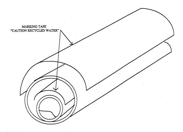
The recycled water sleeve shall be ductile iron. Both pipe and sleeve shall be identified as recycled water piping.
