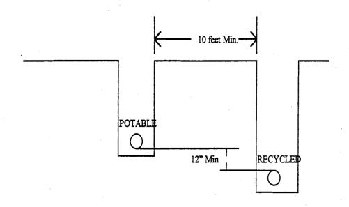
Ten feet of undisturbed soil must exist between recycled water and domestic water piping. Recycled water and Domestic water piping are not to be installed in a common trench with less than the minimum separation. (See Figure 3 for exceptions to the "Basic Separation Rule".)
