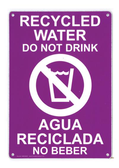
The Recycled Water Sign to be posted at wash-down hydrants, blowoff hydrants, blow offs on strainers and other such facilities, shall measure not less than 8" by 8". The sign shall have a purple background with  $\frac{1}{2}$ " minimum white lettering which reads: RECYCLED WATER – DO NOT DRINK AGUA RECICLADA - NO BEBER.
